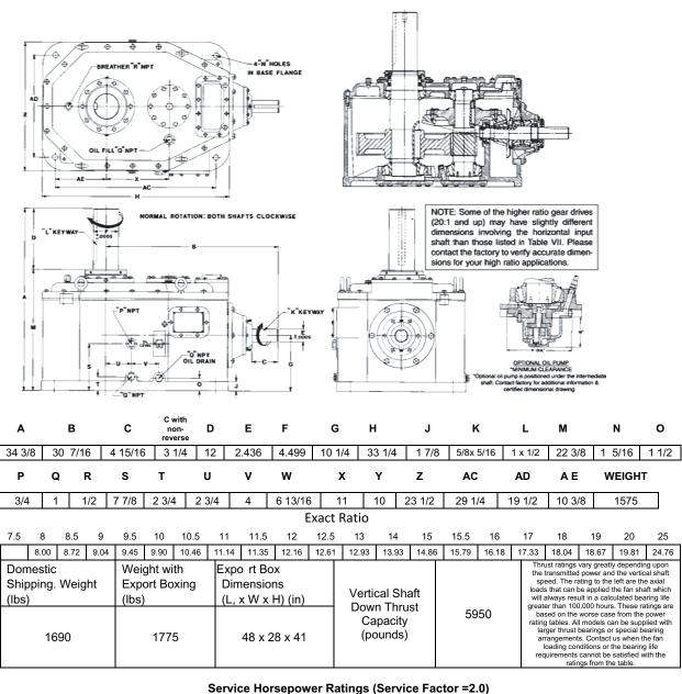
RATIO\* Input RPM 7.5 8.5 9.5 10.5 11.5 12.5 15.5
